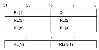
The number of run-level pairs varies from block to block, so a (run,level)=(63,128)=0xfe00 is inserted as a termination code after the final run-level pair in a block.
