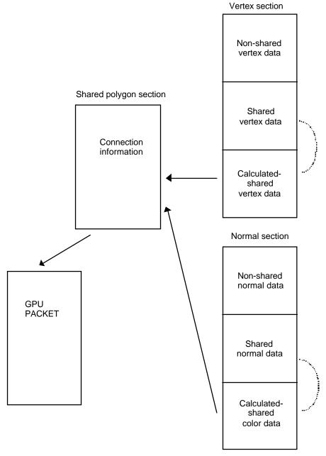
The arrows with the dotted line indicate the processing flow of the PRE-CALCULATION driver. Vertex and normal calculations are performed for each coordinate.
