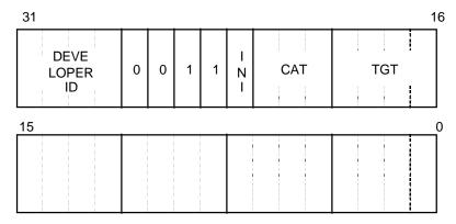
INI: Determines whether a SCAN of the interpolation table section will be performed
