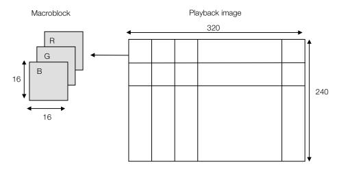
The vertical and horizontal frame sizes should both be multiples of 16. If this is not the case, some additional processing is necessary.
