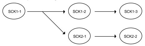
The sequence can be changed to key frame SCK2-1 at any time during interpolation between key frame SCK1-1 and key frame SCK1-2. In this case, a new virtual key frame SCK2-0 is defined at the branch point.
