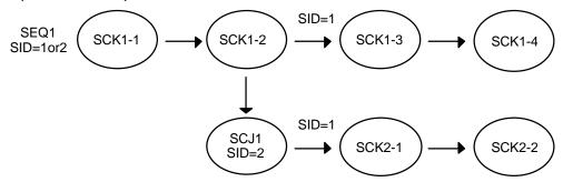
If the SCJ1 descriptor is written in advance and the Sid is 1, this kind of sequence branches to SCK2-1 after SCK1-2. If the information that the Sid is to be set to 0 after the jump is written for the SCJ1 descriptor, the Sid is set to 0 after the jump. Since SCJ descriptors can be arranged in multiple series, individual jump destinations can be specified for various Sids
