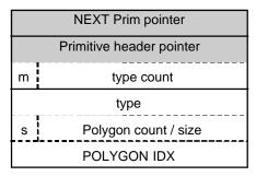
The first three words in a primitive specify the control section. This section is made up of a NextPrim pointer, a primitive header pointer, and a type count. The MSB of the type count(m) serves as a flag indicating whether or not the NextPrim pointer and the primitive header pointer have been mapped. If m=1, the pointers have not been mapped. Conversely, if m=0, the pointers have been mapped.
