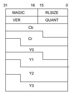
The RL data footer padding (0xfe00) is not included in BS data. So when BS decoding is performed, DecDCTvlc() automatically adds footers to maintain 32-word boundaries.
