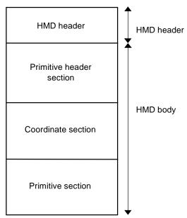
In the example shown above, a coordinate section is included in addition to the required sections.
