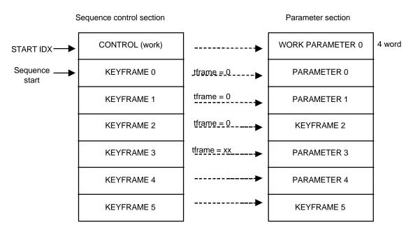
Figure 137: BSPLINE Interpolation
