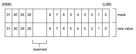
The first word is a mask which indicates the section which changes value and the section which does not change value. 0 is set in the bit which corresponds to the item which will change and 1 is set in the bit for the value which will not change.
