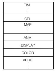
The block is composed of lines assigned key word values.
