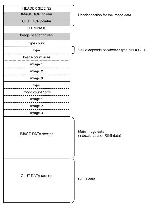
Figure 114: Parameter Memory Area of Image Primitive Driver
