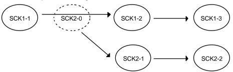
To implement this function, the sequence pointer is set as described below. An area for saving the current parameters is created in advance by entering a DUMMY key frame. This is defined as SCK2-0. Then, SCK2-0 is entered in INTR IDX at the frame at which the sequence was switched. 0xffff is entered in INTR IDX at the next frame. Oxffff prohibits parameter updating. This process enters the current location's parameters in the key frame entity pointed to by SCK2-0.
