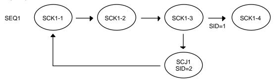
A loop sequence is realized by jumping forward according to a jump descriptor. Looping continues while the SID is 2, and control escapes the loop when the SID is set to 1. The loop can be controlled interactively by rewriting the SID at execution time.
