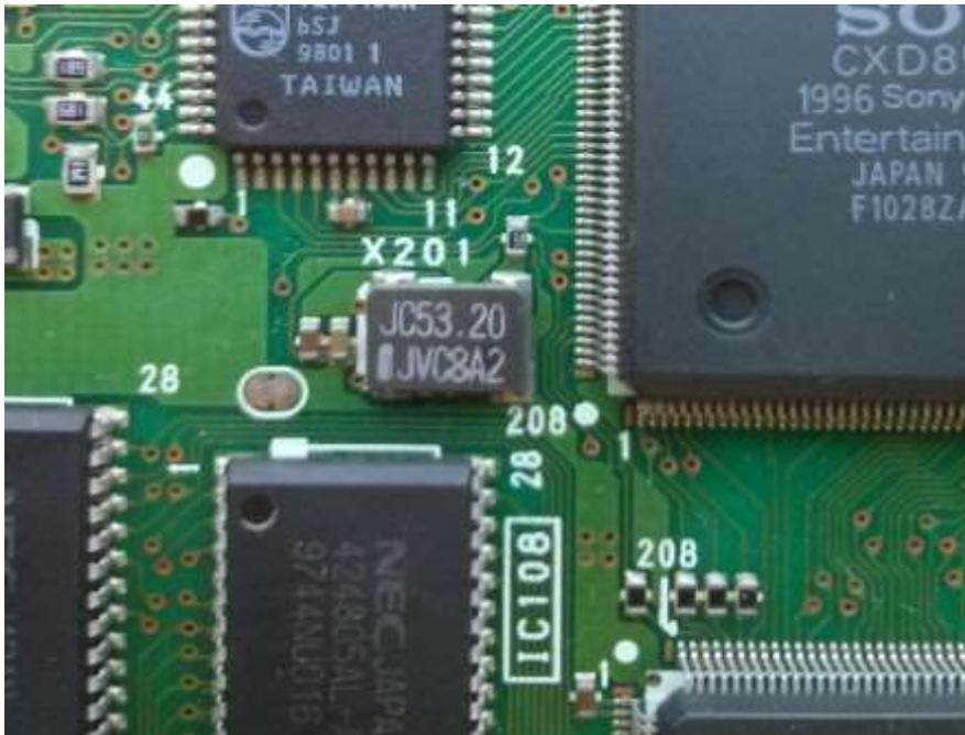
Note that in both cases the reference designation (X201) is the same; it's just the frequency that changes. If you are taking the parts from another PU-18 board (which is what this guide is assuming) , the locations are shown in the next two photos:
