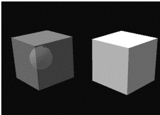
NOTES: Making a texture polygon (provided with applied texture) semi-transparent requires that the TIM utility has been used to set the texture semi-transparency control (STP) bit at 1.
