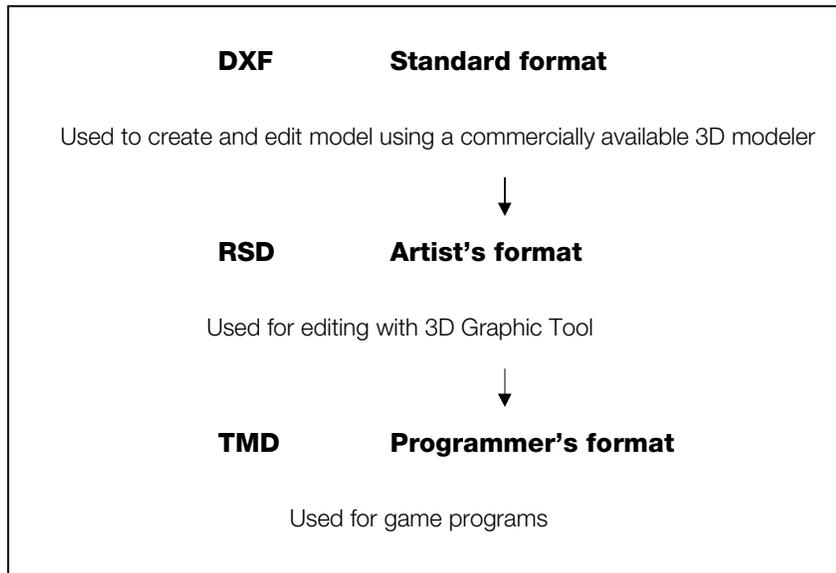
To create characters and buildings used for a 3D game, you perform modeling with a commercially available 3D modeler, convert format using the 3D Graphics Tools, add material data, and finally create a file that can be utilized by a program.
