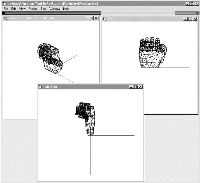
The hand shown on the screen has the following hierarchical structure. (It is shown in General, Left Side, and Front windows in Figure 6-31.) As in the example of the robot arm, the joint of each finger is expressed as origins so that the movement may be transmitted from the root of each finger to the tip.
