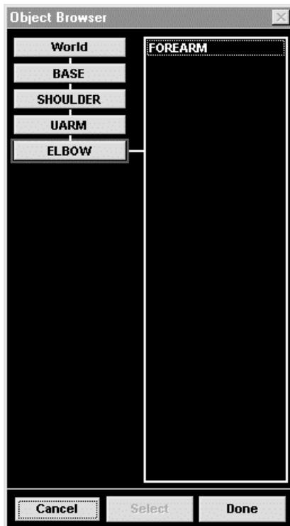
On the left, the World, Base, Shoulder, UArm, and Elbow buttons are located from the top to the bottom in that order. The red frame of the Elbow button indicates that it is currently selected. They constitute the hierarchy of the objects above Elbow. The left field indicates Forearm, which is the child of Elbow.
