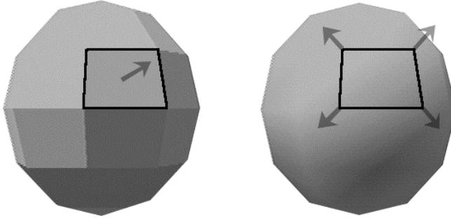
Smooth shading for a cube is difficult to understand. Make a try using a curved-surface model, such as a ball. (Sample data in `SPHERE.DXF` is sphere data.)
