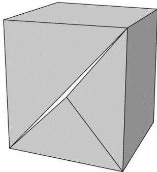
Also, avoid coupling two 3D models prepared independently from each other by mating the surface of one polygon to that of another as shown in the figure below. No problem will arise if the vertex coordinate values are just the same. Otherwise, a gap will be created. The two coupled surfaces are useless polygons that are never seen.
