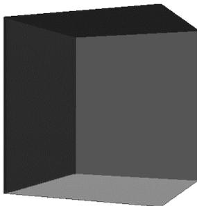
DXF does not allow direct description of "front and back of a polygon". The front is determined according to the order of description of vertices of a polygon. Depending DXF, this order may be reversed. In such a case, the front and back can be exchanged by specifying this option. The vector that expresses the direction of the front of a polygon is called a normal vector.
