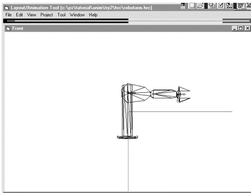
Before selecting the elbow, select the Origin icon on the tool palette, to restrict the object of manipulation to the origin. (While the origin icon is selected, there is no fear for selecting a model or camera by mistake.) Then, select the parallel translation icon to move the origin to the position of the arm without rotating it.
