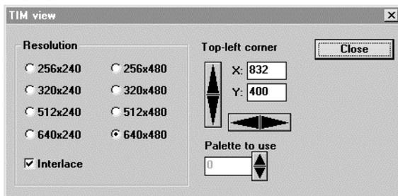
Using this dialog box, you can specify the image resolution of Artist Board, and display area start position on VRAM. You can scroll the image up and down, and to right and left by changing the display start position.
