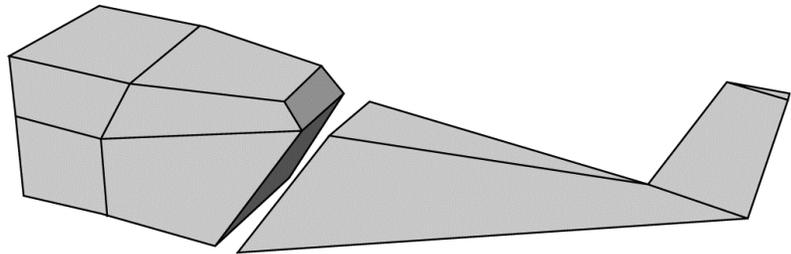
Using the modeler, you should extrude an existing surface or side to create a new surface instead of inserting new vertices to a middle point of a side, or to any other position (even if you can do so). This function is one of the fundamental functions of the 3D modeler, which is called Extrusion.
