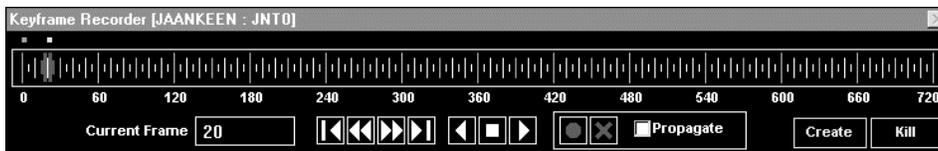
In a similar manner, move the slider on Keyframe Recorder to the "40" position, and rotate the hand around the Z-axis by 60 degrees from the original position to get the same pose which existed when TE.HRC was opened. This is the starting position for lowering of the hand for the second time.
