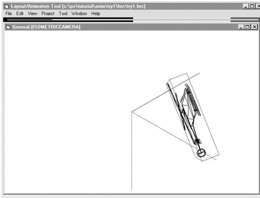
This is the rotation of the object. The center of rotation is always the center of the bounding box. In the first method, the direction of the rotation axis always changes. In the second, it is constant until you release the mouse button.
