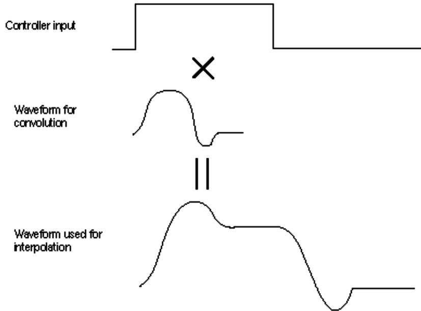
The program becomes simple if convolution is employed to respond to controller input. In the case of MIMe animation which does not resort to the controller, the control waveform is directly used as a weight factor.
