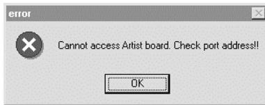
In this case, correct the `ABOARD.INI` file using the `ABOARD.EXE` tool, or change the address of the board itself so that the values of these addresses may become the same.
