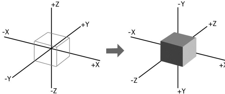
The front and back of a polygon are inverted each time you exchange Y-Z axis and + and - once using this option. If you specify correctly, you do not have to specify the `-back` option.
