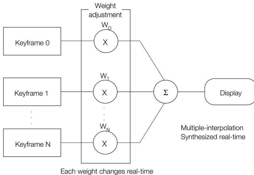
NOTES: The concept of MIMe is not restricted to vertices. It can be applied to variations, such as normal, angle, and UV coordinates of a texture. For simplicity, only vertices are discussed in this section.
