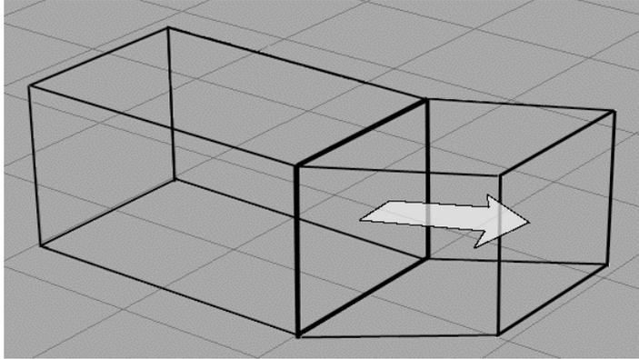
Otherwise, a fundamental shape, such as a rectangular parallelepiped, may be divided into small polygons, and then the shape may be modified by moving the vertices.
