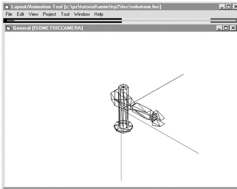
Open `c:\PSXGRAPH\TUTORIAL\ANIM\TRY2`, and then open `ROBOTARM.HRC`. A robot arm appears on the screen. The same image can be obtained if you assemble parts, such as the arm and mount, to get the same layout. However, it is too great a burden to do so each time you move the arm. To move the lower arm and hand according to bending of the elbow, you may use the hierarchical structure.
