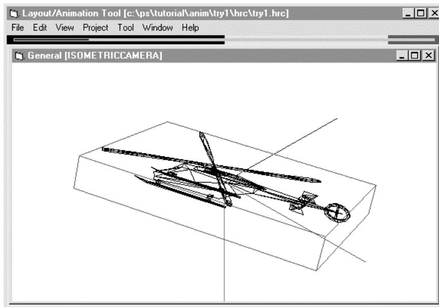
This finishes enlargement and shrinkage of an object. The first method is proportional enlargement and shrinkage not dependent on the direction. The second method is enlargement and shrinkage having a direction. The scale factor for enlargement and shrinkage is 1/4096 time to about 8 times (8 times to 1/4096 time) because of the restrictions imposed by PlayStation.
