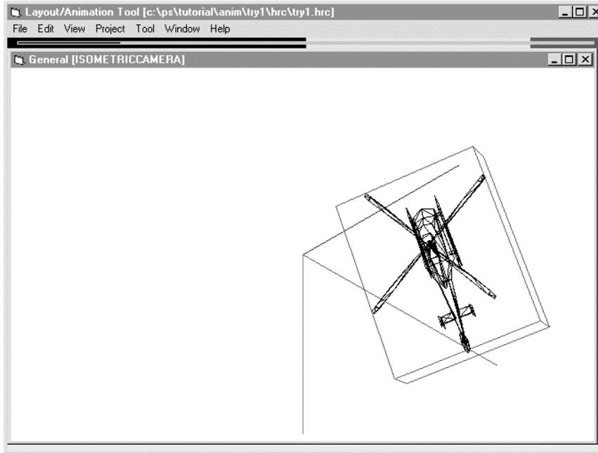
Then, put the mouse onto a line of the bounding box, and drag it. The bounding box rotates around an axis parallel with the line. Release the mouse button. The helicopter is displayed in the same posture as the bounding box. This method may be used to adjust the posture.
