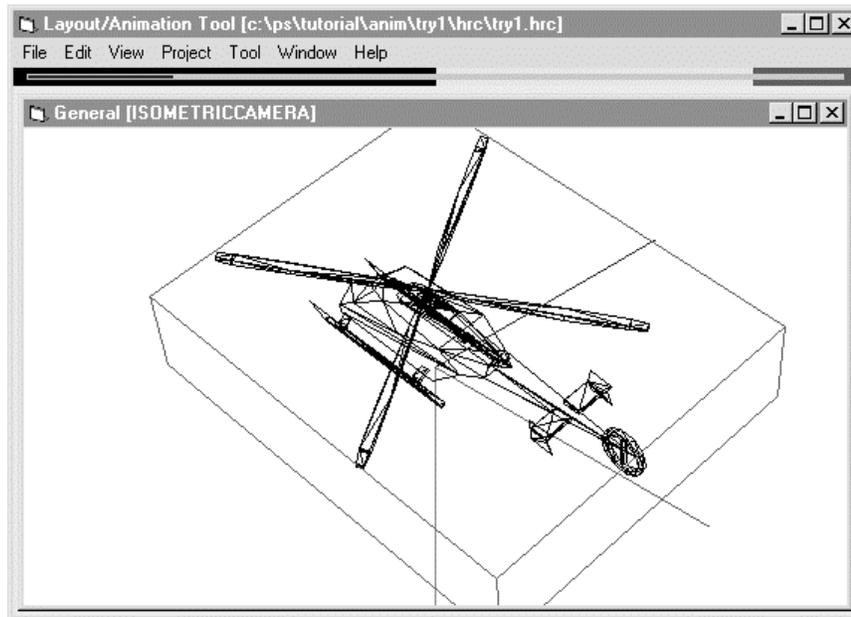
While holding down the Ctrl key, put the mouse cursor to a plane of the bounding box, and drag the bounding box. If you drag the plane away from the bounding box, the plane is drawn out and enlarged. If you bring it near the center, the object shrinks as if it were crushed by that plane.
