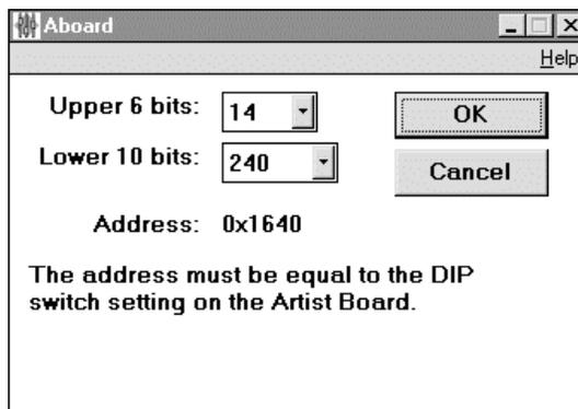
Upon the first startup of ABOARD.EXE, 0 x 1340 is displayed as the address. This is the factory set default for the artist board. If the I/O address has been changed by the dip switch on the board, use this application to modify the address setting.
