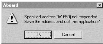
This means that the artist board has not correctly reacted to the set I/O address.
