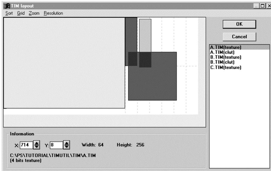
You will see the screen display shown in the figure above. It is difficult to precisely put A.TIM onto the texture boundary using the mouse. There are two methods to get around the difficulty. One method is to set numerical values in X and Y for the data area to determine the position. The other method is to utilize the grid function. We will use the second method because it is more convenient.
