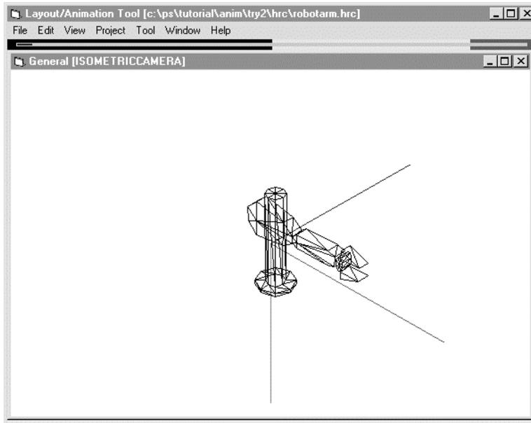
Open c:\PSXGRAPH\TUTORIAL\ANIM\TRY2, and then open ROBOTARM.HRC. A robot arm appears on the screen. The same image can be obtained if you assemble parts, such as the arm and mount, to get the same layout. However, it is too great a burden to do so each time you move the arm. To move the lower arm and hand according to bending of the elbow, you may use the hierarchical structure.
