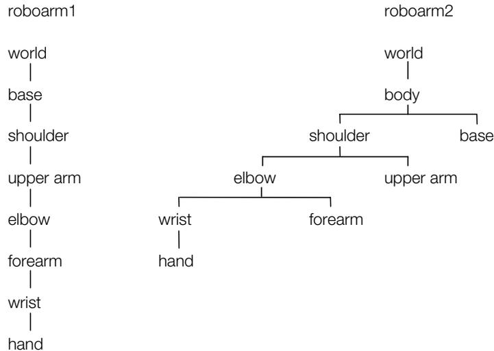
If a hierarchical structure contains a model that is likely to be enlarged and shrunk, it is essential not to create a child or grandchild below that model in the hierarchical structure.
