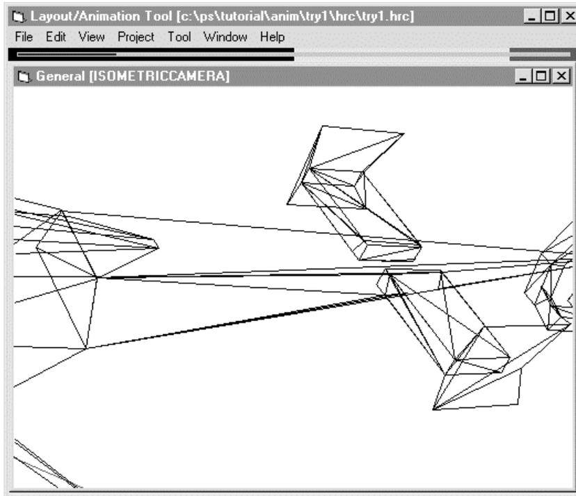
Holding down the Ctrl key, strike the right cursor key. The direction changes only a little. To fine-adjust the direction of the camera, strike the right or left cursor key while holding down the Ctrl key. Each time you strike the cursor key with the Ctrl key held down, the camera rotates by one degree.
