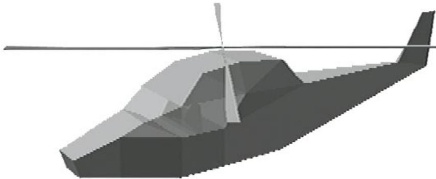
This helicopter consists of two objects: body and rotor. They can move independently, and hierarchical relations between them can be defined. For these purposes, however, each object must be created as different RSD data. (In other words, the parts that move in concert with each other should be defined as one object and coordinated into the same RSD even if they are apart from each other.)
