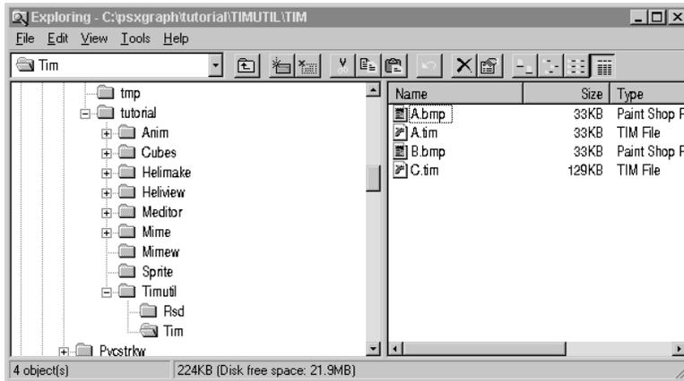
Select a .tim on the window using the left button of the mouse. While holding down the left mouse button, drag it to the window for TIM Utility. When the mouse cursor is put into the window for TIM Utility, release the button. Now, A .TIM is opened.
