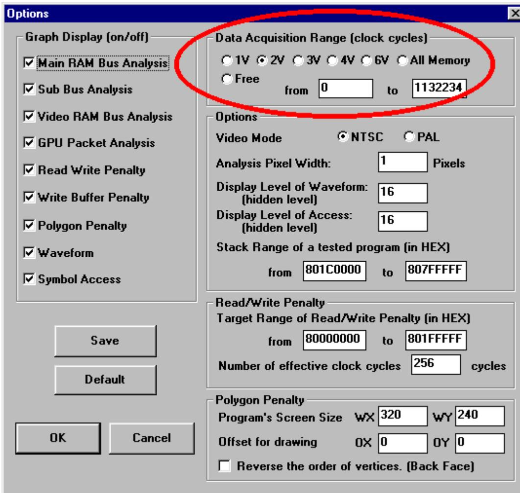
Clicking one of the radio buttons the corresponding clock range. The All memory radio button corresponds to the measurement of about 7.4V blanks (NTSC) or about 6.2V blanks (PAL). Increasing the measurement range enables the analysis of a larger amount of data, but the time taken for data read and hard disk consumption increase accordingly.
