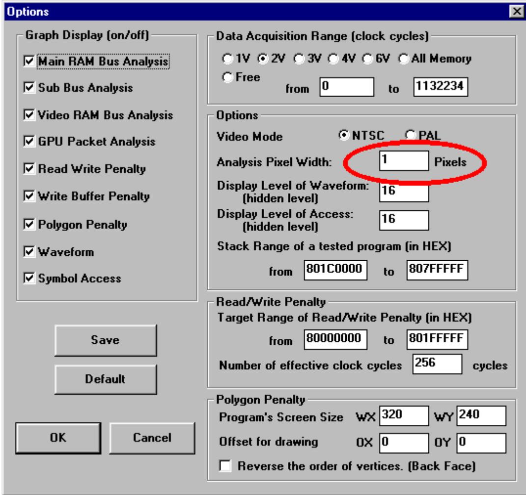
This option is provided to make the histogram easier to understand by changing the pixel width. The default pixel width is one pixel. If, however, it is changed to five pixels, the analysis display will change as shown below.
