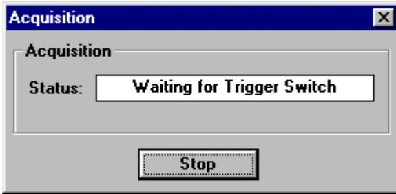
Press the trigger switch when the scene to be measured appears. Data read starts immediately, provided there is no trigger condition other than the trigger switch, as in this example. If trigger conditions other than the trigger switch are specified, the data to be measured once all the conditions are satisfied starts to be read when the switch is pressed.
