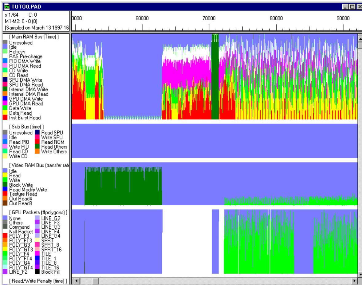
This display is so fine that colors mix with adjacent colors making identification difficult. Therefore, select "Options..." from "Setting" menu and change "Analysis Pixel Width" in the Option dialog box.
