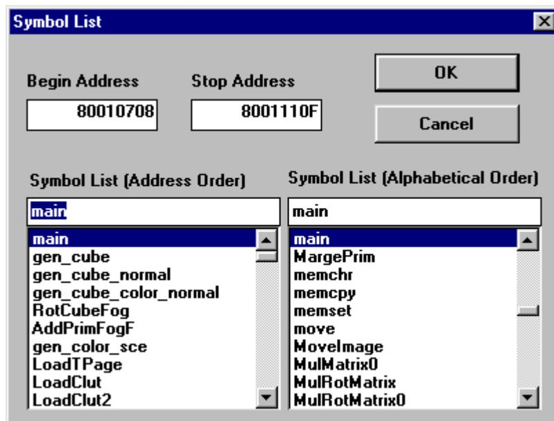
Note: Care is required when you use the address of a function as a trigger condition, as the Performance Analyzer cannot observe the functions in the instruction cache. This is because it can measure the status appearing on the bus, but cannot measure the status within the CPU. Therefore, while it is
