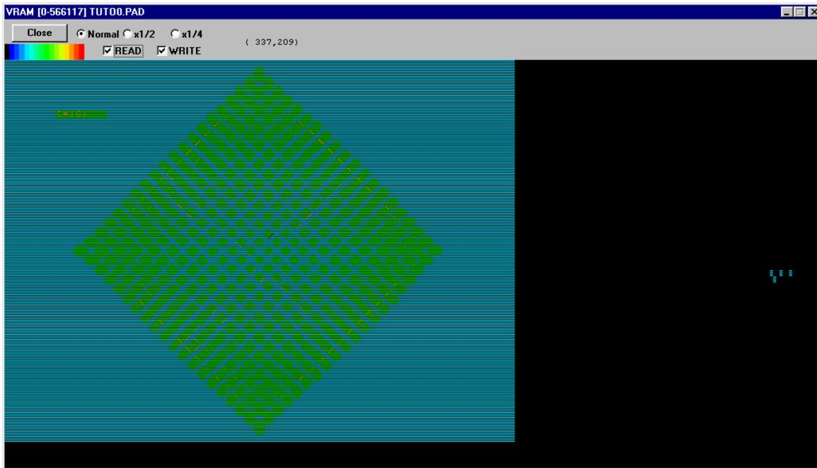
The accessed pixels are displayed in palette colors according to the access frequency (Low: Blue, High: Red). It is also possible to display read and write accesses separately by selecting the Read/Write checkbox accordingly. This makes it possible to read the sections where polygons are drawn, the texture and CLUT as well as to identify the sections to be subject to semi-transparent processing.
